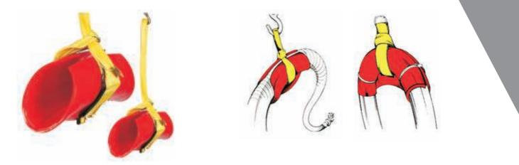
A PUHB Hose Saddles is a polyurethane saddle designed to suspend hoses. Each model comes complete with its own UV treated polyester sling which is fastened in a choker position. The PUHB Hose Saddle is designed to accommodate the manufacturers' minimum bending radius to protect hose from kinking and prolong the life of the hose.
